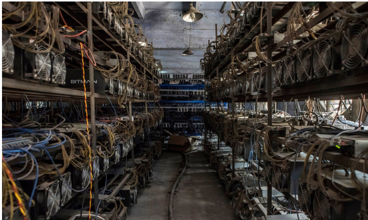
Figure 9: Racks of machines mining Bitcoins and Ether at a server farm in Guizhou, China, June 2017. Current hash rate estimated at 10 million trillion SHA256 hashes per second! Over USD1.1 billion of electricity consumed annually, about the use of Ecuador. Sources: photo Gilles Sabrié for The New York Times, https://blockchain.info/charts/hash-rate , https://digiconomist.net/bitcoin-energy-consumption
